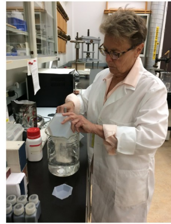
Chris mixes a solution of gellan gum to make a poultice for stain removal. Photo credit: The Royal Ontario Museum.
